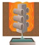
De-Waxing & Shell Backing
